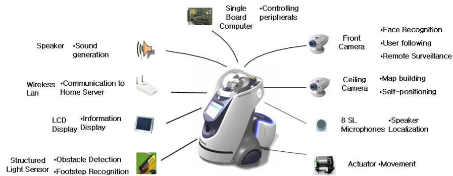
Fig. 1. HW Components of SHR100
